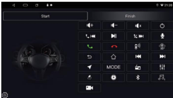
The positive and negative electrodes of the steering wheel control wire of the original car and the positive side of the machine control wire are connected to the negative electrode. Press the steering wheel keys in turn, and record the order, click on the corresponding function settings to save the settings.
